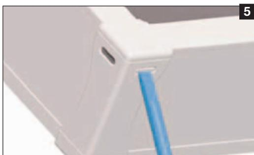
According to the on roof installation break out the two draining slots on each of the two lower left and right corners of the collector frame. Use a slotted screwdriver for this and put it on bottom edge of the draining slots to break slots out.
