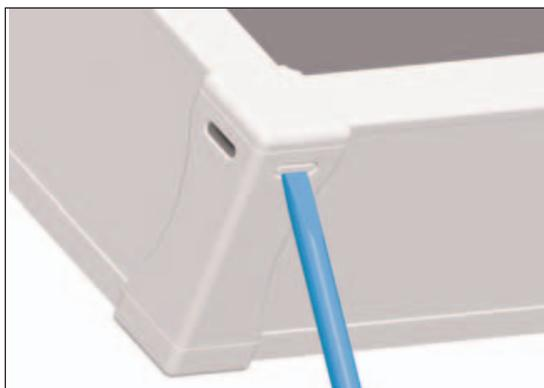
5. Punch the two drainage holes at each bottom corner of the collector, according to how it is mounted, with the aid of a slotted screwdriver. To do so, punch at the bottom edge.
